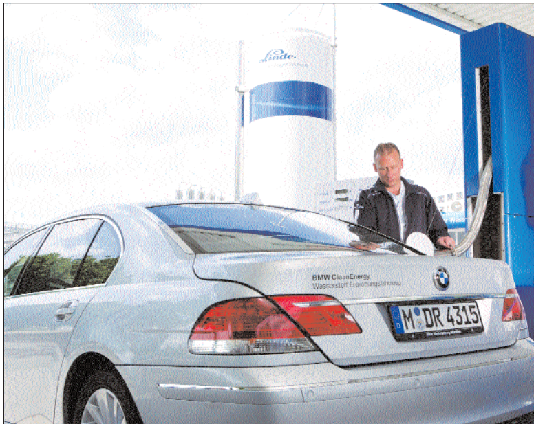
BMW's Hydrogen 7 series burns hydrogen in an internal combustion engine
